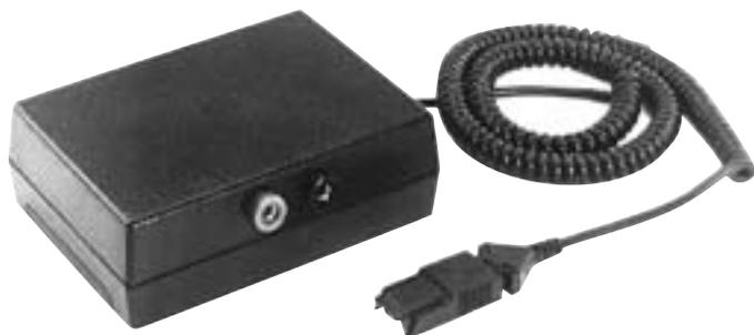
The MOD400R Field Sensitivity Test Module can be used with any standard DC voltmeter or multimeter to check the sensitivity range of System Sensor's detectors (satisfies NFPA 72 requirement for sensitivity testing).
